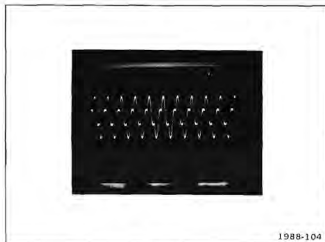
Figure 4-6. Current waveform at T1230 for normal inverter operation at line voltage of 115 V.
